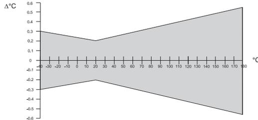
Temperature dependence of electronics typ. ± 0.005°C/°C
