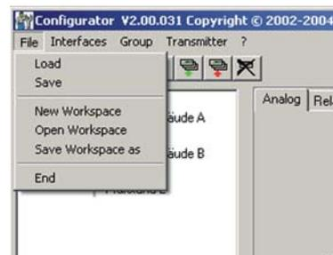
**Load:** Loads a file with a saved transmitter configuration.
