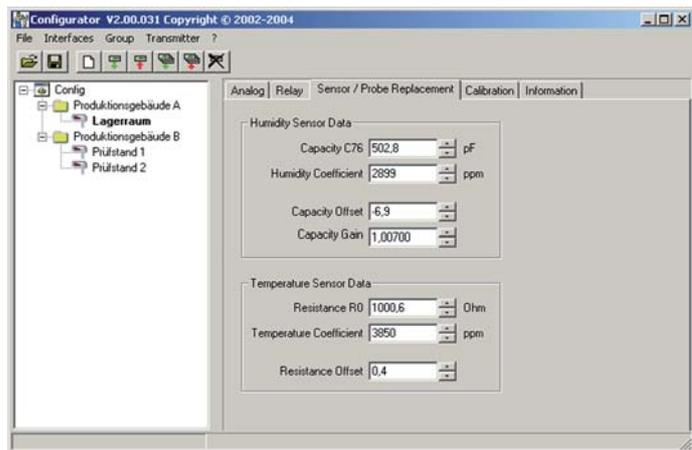
In case of sensor or probe replacement, the characteristic values for this sensor/probe must be saved in the transmitter to ensure the transmitter will operate within the specified accuracy range.
