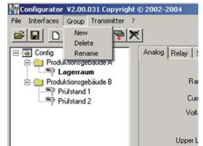
The icon "Group" provides the option of combining transmitters in groups. A group may consist of transmitters used in the same application, for instance assigned to a building.
