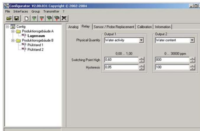
Used to set both optional alarm outputs.
