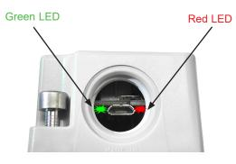
Green LED flashing = Normal operation
