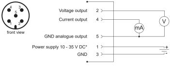
\*The supply circuit must be fused with  $\leq$  8A
