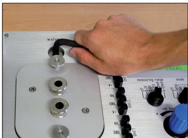
Enter the humidity value in the HUMOR 20 display and the reference value of the chilled mirror dew point meter into the corresponding software fields and confirm your entries by pressing "Store".
