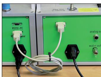
Establish a serial connection between HUMOR 20 and the automatic calibration module. Connect "RS232-Humor" on the automatic calibration module with "RS232" on HUMOR 20.
