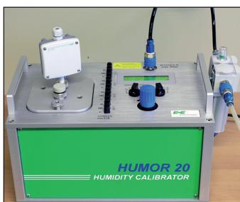
Because of the operating principle, HUMOR 20 has a slightly higher temperature than ambient. During the measurement process, make sure that the probe temperature can adapt to the temperature of the measuring chamber.
