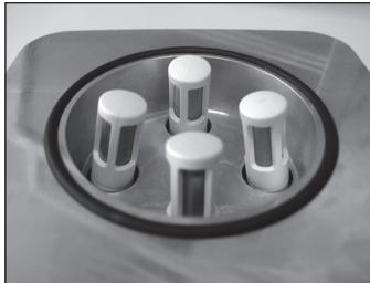
3. Seal the openings of the feedthroughs not in use with the supplied plugs.
