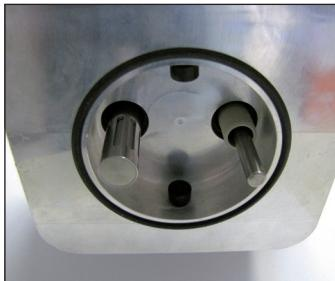
1. Plug both air vents of the cover of the measurement chamber with the plugs supplied with the adapter (see left picture).
