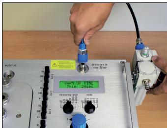
Attach the oil separator / filter set to the side of HUMOR 20, on the bracket, and establish a connection to the input "Pressure in".
