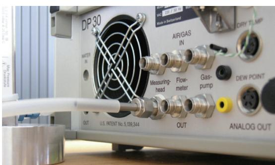
2. In order to acclimatise the measurement setup to the ambient temperature the HUMOR 20 should run an additional two hours after warmup.
