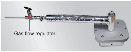
1. Fit the calibration cover (available on request from E+E Elektronik) and connect with the chilled mirror dew point meter.
