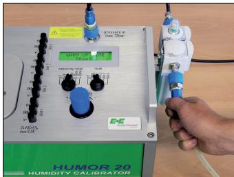
⚠ Connect the pressurised (min. 8 bar) compressed air line to the filter set. A pressure less than 8 bar can cause leakage at the filter set.
