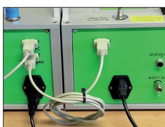
Establish a serial connection between the automatic calibration module and the PC/notebook.
