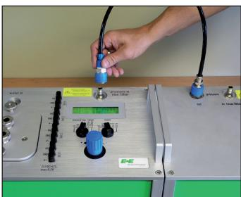
Establish a compressed-air connection between HUMOR 20 and the automatic calibration module.
