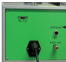
On the back panel of the HUMOR 20 sits a 4-pole connector with the label "analog out".
