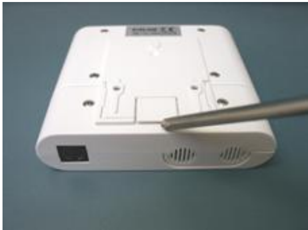
Illustration: Removing the Back-Plate
