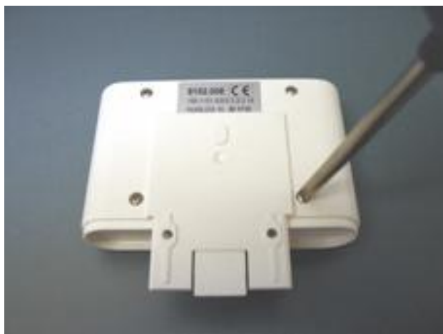
Illustration: Opening the HUMLOG 10 to change the battery
