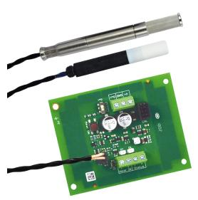
The high-quality, flexible probe cable up to 3 m facilitates mounting of the EE1900. The electronics board is available in two sizes, for easy integration into existing climate chambers and other machines.
