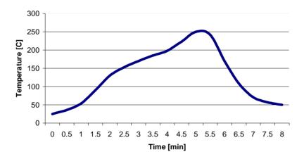
The exact profile must be optimized to the corresponding SMD soldering system. Make sure that the maximum temperature of 250°C (482°F) is not exceeded for more than 3 minutes, and that the specified time is generally adhered to. The entire time duration for soldering is not allowed to exceed 10 minutes at temperatures > than 180°C (356°F).
