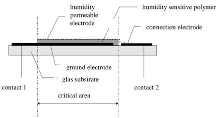
This determines the **critical area** of the active sensor surface, which must be handled with extreme care to avoid **contamination and damage (such as flux residue, solder splashes, scratches, fingerprints, etc)**. Contamination and damage outside of the critical area impair the measurement function only in exceptional cases.
